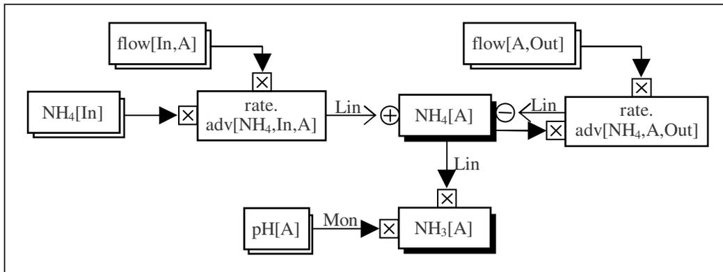
Figure 11: The resulting model for the interaction of dissociation and advection
