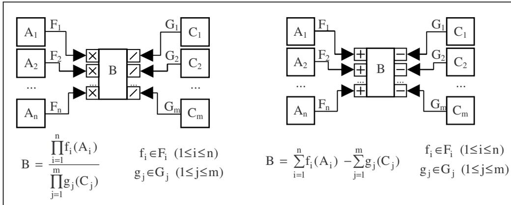
Figure 4: The basic elements of the influence diagrams, with completely multiplicatively and additively decomposed influences
