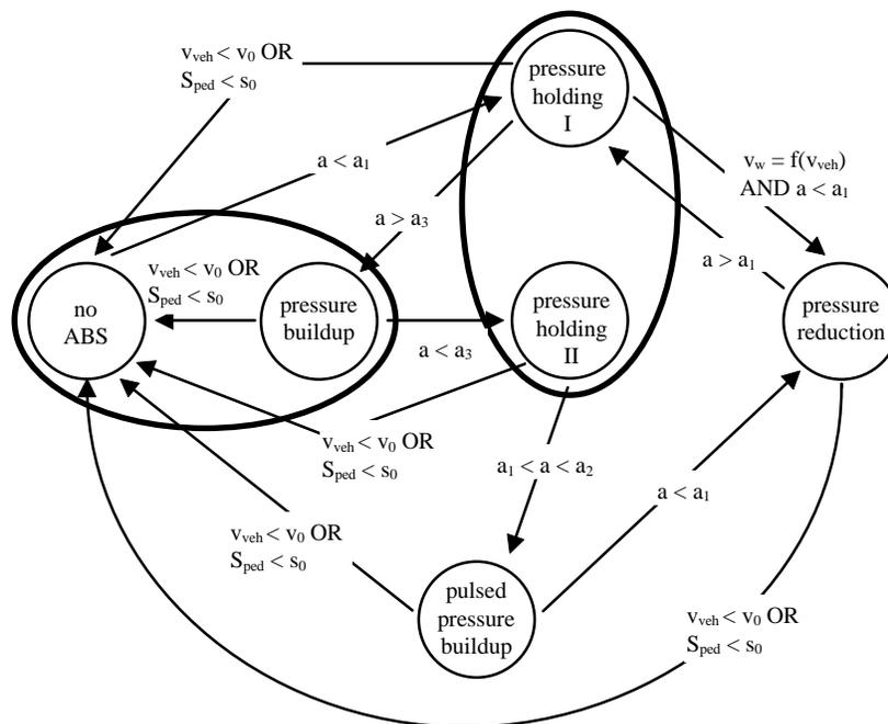
Figure 3: States and transition conditions of the ECU
