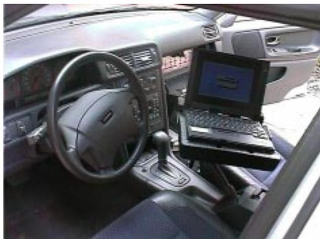
Figure 3: View of the Volvo Demonstrator Car showing the notebook connected to the ECU. The glove compartment (behind) contains the switchboard for controlling the built-in faults.
