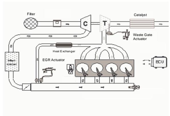
Figure 8 Guiding application: Air delivery system
