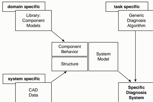
**Figure 3: Automated generation of model-based diagnostic systems**
