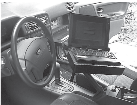
Fig.4: View of the Volvo Demonstrator Car showing the notebook connected to the ECU. The glove compartment (behind) contains the switchboard for controlling the built-in faults.
