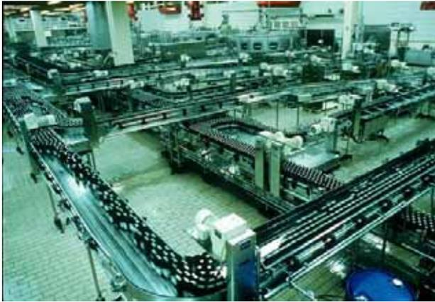
**Figure 1.** Conveyors of a bottling plant for returnables
