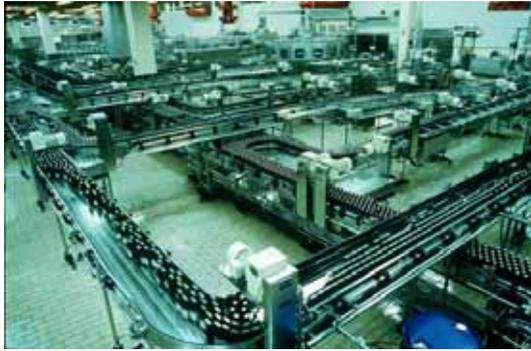
**Figure 1.** *Conveyors of a bottling plant for returnables*
