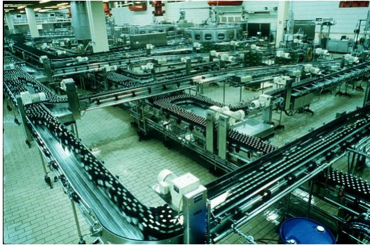
Figure 1. Conveyors of a bottling plant for returnables
