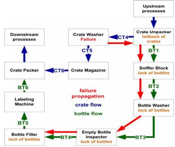
Figure 5. Failure propagation (red arrows) via sub-branch of production line causing a lack of bottles at the Filler
