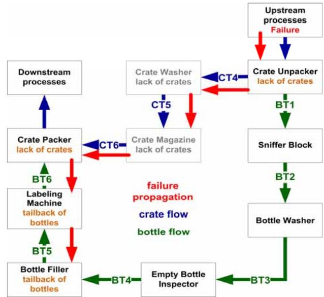
**Figure 7.** Failure propagation via sub-branch of production line causing a tailback of bottles at the Filler
