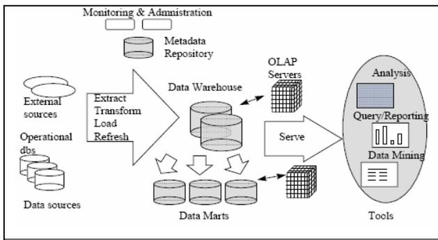
Figure 1. Architecture of a generic data warehouse system.
