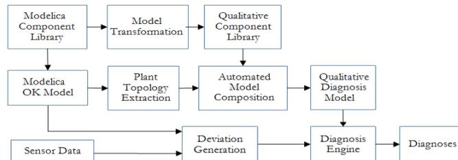
Figure 2. The workflow: from Modelica model to diagnosis.
